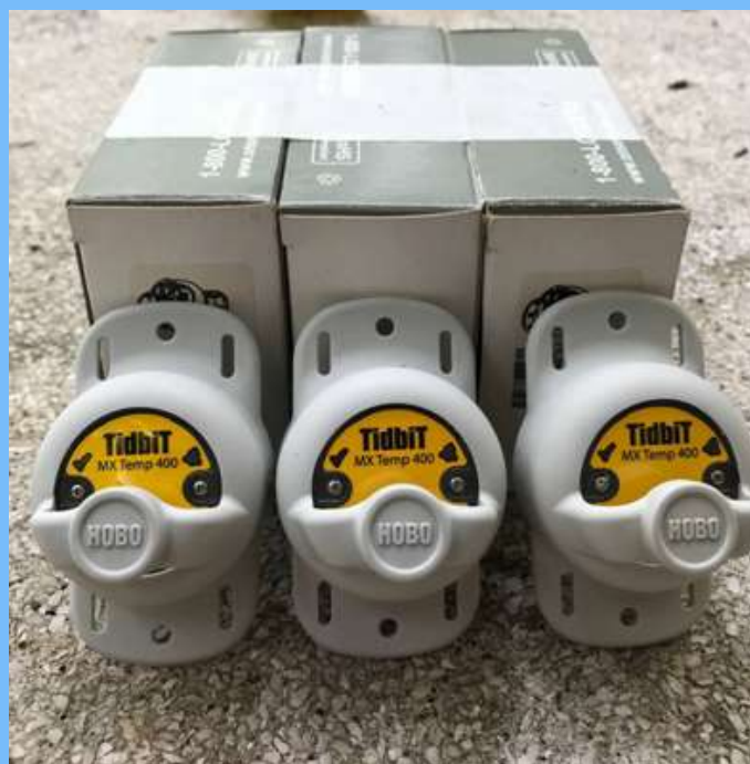
Figure 3. The team conducting post-emergence inspection (PEI; top), in which the HOBO MX TidbiT 400 logger placed in some of nests to track incubation temperature was removed (bottom).
